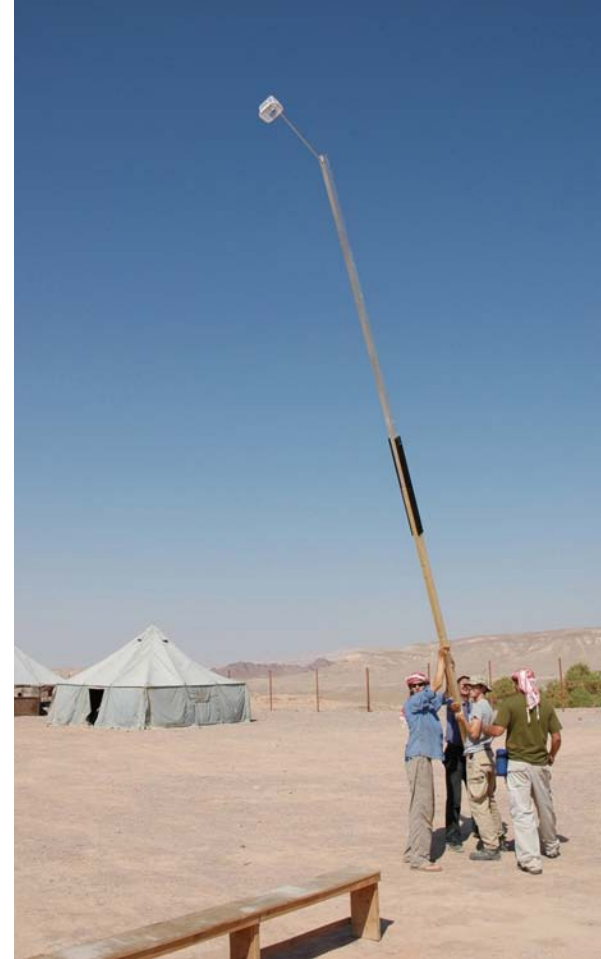
'Aerial Photography' system used in 2004. A small digital camera was attached to the end of the stick and raised over the 5 x 5 meter excavation trench. Photos were taken and were downloaded to a GIS to be combined with architectural drawings.
