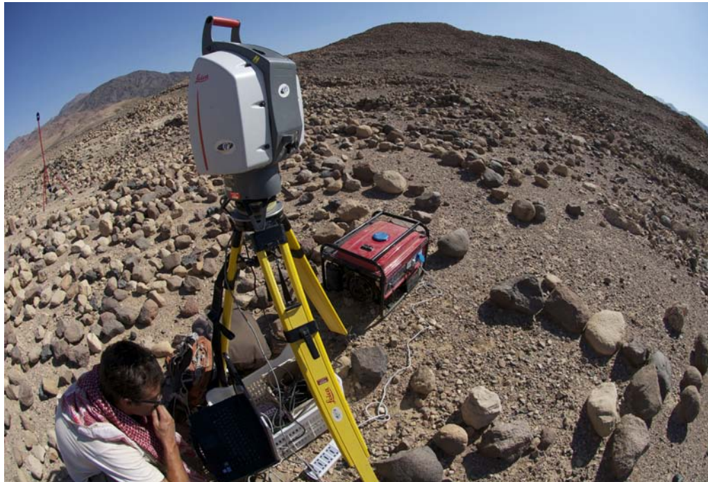
Student helps monitor the LiDAR (Light Detection and Ranging) laser scanner at Khirbat Faynan (Biblical Punon) in Jordan. LiDAR enables researchers to collect billions of geo-referenced data points (accurate to +/- 1 cm) to create 3D maps and models of ancient sites and their environments.
