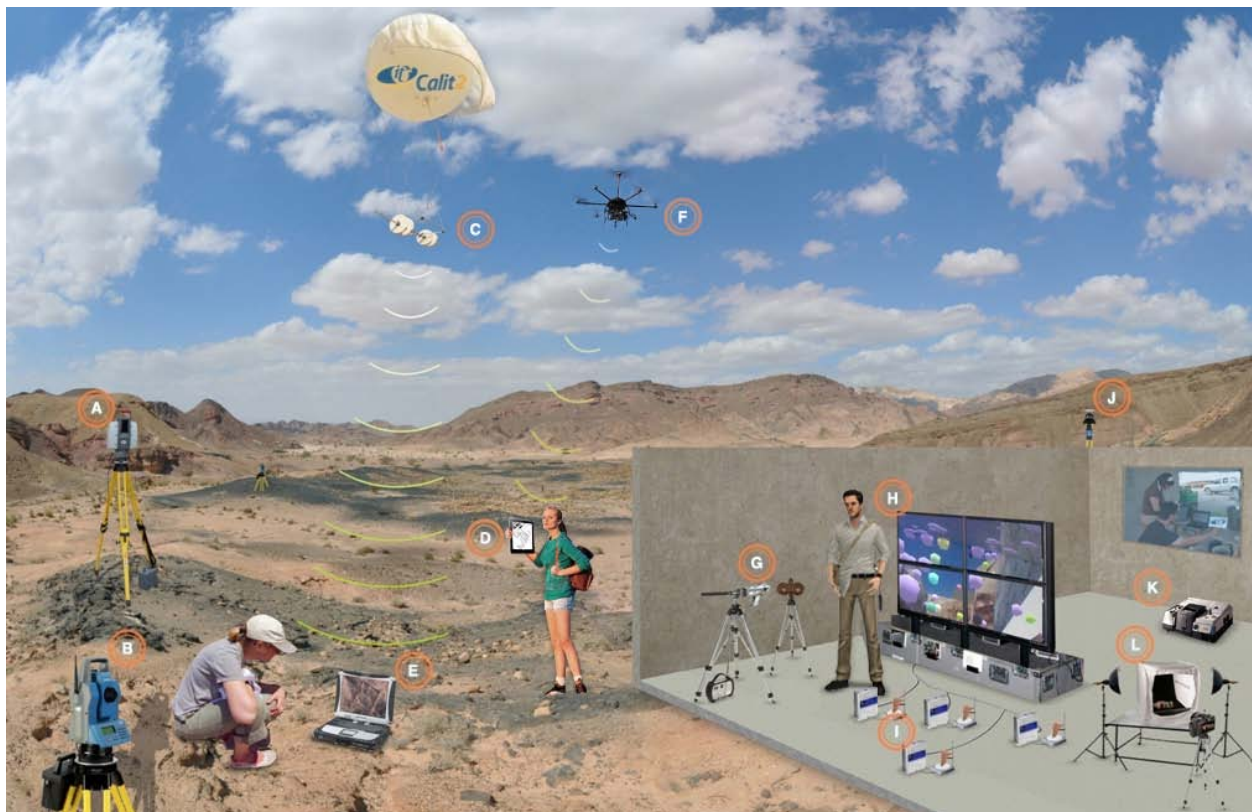
Model of the 2012 Cyber-Archaeology field and lab methods deployed by the UCSD-Calit2- team in Jordan’s Faynan district. In the field: A) LiDAR Scan-Station 2; B) Leica Reflectorless Total Station; C) Helium Balloon with gimbal platform for HD photography, D) iPad or Tablet computer for ArchField and OpenDig recording, note – operator has WHS British trowel; E) Tough-Book Laptop Computer for wireless control and viewing of balloon cameras; F) Octocopter aerial imaging platform. In the lab: G) Portable Bruker XRF; H) 3D Opti-portable visualization platform; I) NextEngine 3D scanners; J) RTK-GPS; K) Nicolet FTIR spectrometer; L) Digital HD photography studio.
